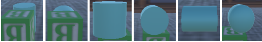
Figure 10: Sample of misrecognized objects. From left: cylinder misrecognized as cube (1), and capsule (2), cylinder misrecognized as cube (3), sphere (4), and capsule (5), and capsule misrecognized as sphere (6).
